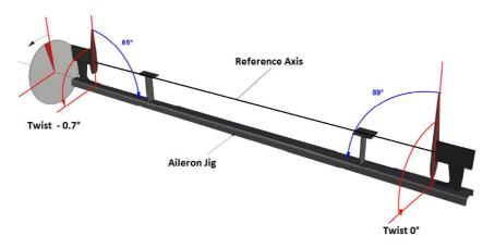
Within this Manual we will also supply the jigs drawings including pictures of our jigs which have been realized in our plan... of course our jigs have been realized in steel which is the material that we usually manage, however you can easily realize yours in wood material as long as the reference axes and distances comply with the ones provided.
